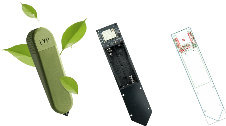
Figure 2: End-to-end product: PCB design, firmware, native app, and 3D design for a connected device
